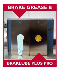
**TEST:** Braklube Plus Pro and two other brake greases were smeared on a metal plate that was placed vertically and heated up to +240°C, simulating the working of brakes.
